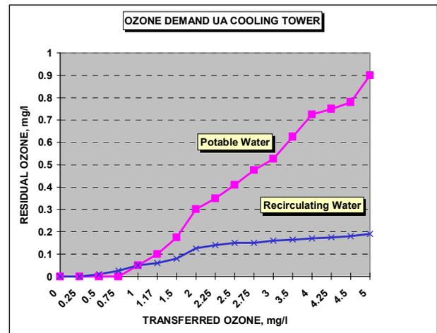
The amount of ozone required to satisfy the demand exerted by the potable water makeup and the recirculating water to produce an ozone residual of 0.1 mg/l is given below in Table 3.
